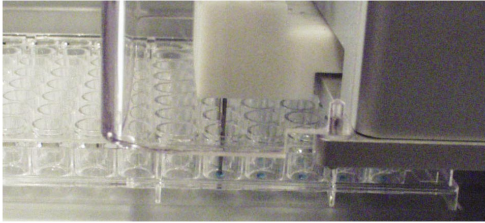
Photo 1: Side View of the Quad-Z 215 Dispensing 1- \mu L Droplets of DMSO into an Empty Microplate
